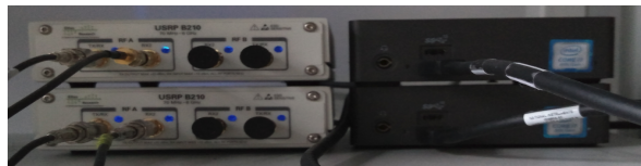
Fig. 1: OAI testbed with two small form factor PCs and two B210 USRP.
